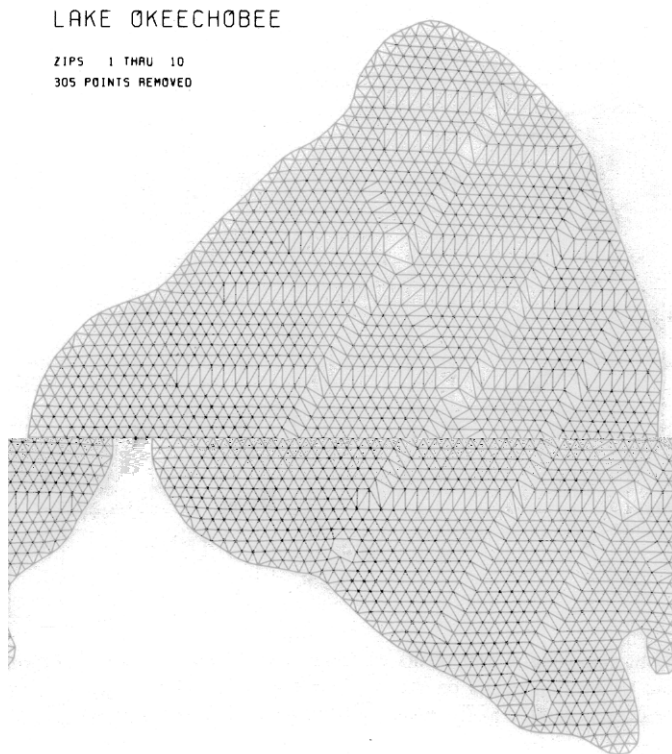
FIG. 9. Ten rows of points have been removed from the region indicated by the contour in Fig. 7, and neighboring points in the vicinity of the cuts have been respecified.
